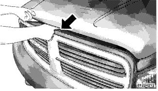
To prevent possible damage, do not slam the hood to close it. Use a firm downward push at the center front edge of the hood to ensure that both latches engage. Never drive your vehicle unless the hood is fully closed, with both latches engaged.
